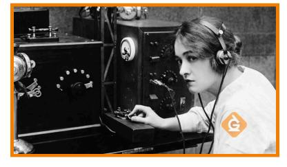
was invented. This machine sent the earliest text messages through a pattern of long and short beeps that correspond to letters and numbers. One person would send the message using the Morse code machine, and then another person would decode the message into letters and numbers. The information traveled as electrical signals across telegraph lines.
