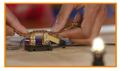
Examples of insulators are wood, rubber, plastic, ceramics, and glass. Different combinations of conductors and insulators can be used to control the flow of electricity. For example, wires in our electronic devices are usually copper wire wrapped in a plastic coating. The copper wire conducts electricity, and the plastic coating prevents the electrical energy from being transferred to another conductor.
