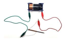
6. Check again to see if the nail is magnetic. Does it attract the paper clips? Record how many paperclips you can pick up with your electromagnet.
